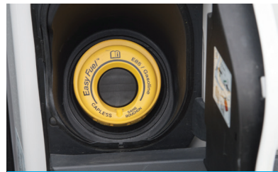
Encased capless fuel filler
